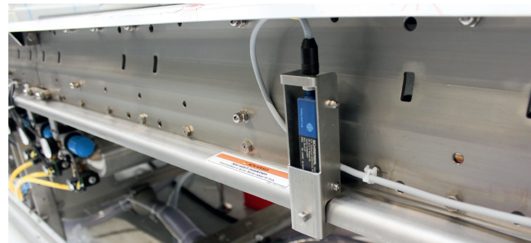
open frame profiles with monitoring of side panels
