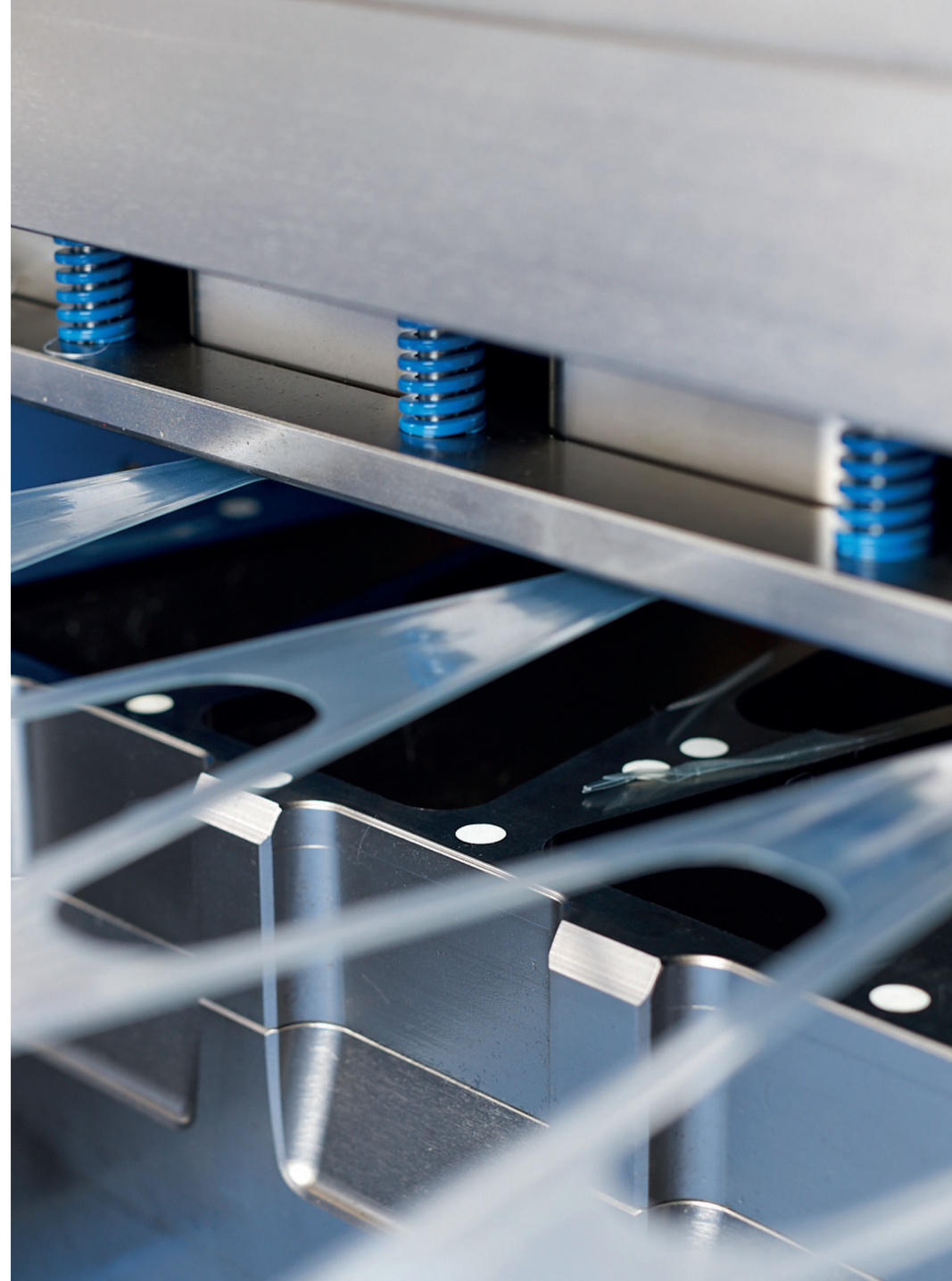
complete cut punch for individual packaging shapes
