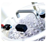
leak tester will be evacuated by injector (rondo) or vacuum pump (quarree). By reducing the air pressure in the leak tester the pack blows up. In case of leaks in film or sealed seams bubbles raise up from the defect spot. After the non-destructive test, faultless packages can be regularly used.
